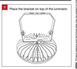
Place the driver back and screw the bracket together
