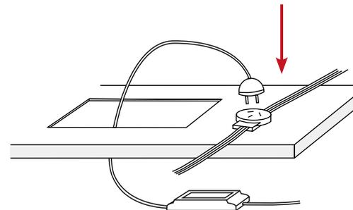
**4** Lift the springs upward to ensure the luminaire can be installed into the mounting hole.
