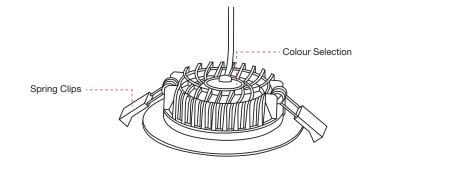
Only adjust CCT switch (located inside rear of luminaire) when luminaire is powered off. CCT switch illustration is shown below.
