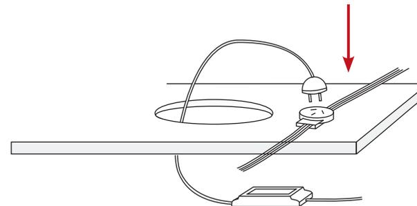
**4** Lift the springs upward to ensure the luminaire can be installed into the mounting hole.
