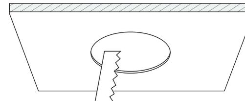
To maintain IP65 rating on XDRL10, ensure that the luminaire is installed on a flat, level ceiling and that the luminaire has an adequate seal to the mounting surface.
